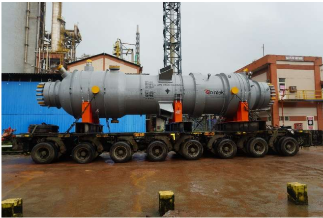
HP Stripper unloaded from vessel and transported by road to PPL, Mangalore
