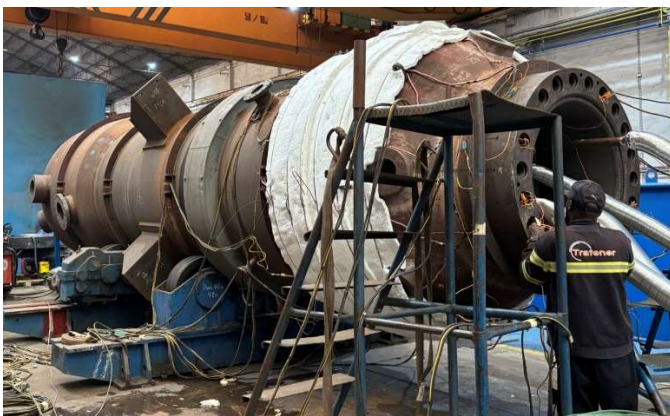
Local PWHT with special Air-cooling header arrangement
