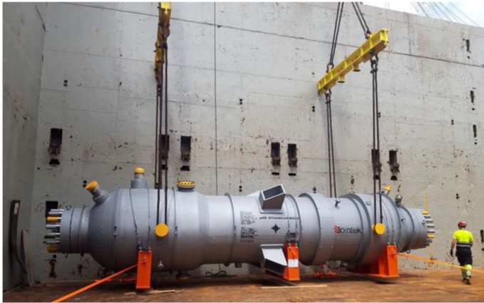
Stripper loaded to vessel for transportation
