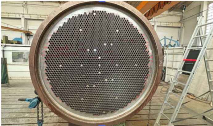
Tube sheet after tube insertion and before channel shell assembly
