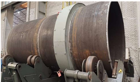
Shell courses with Expansion Bellow during fabrication
