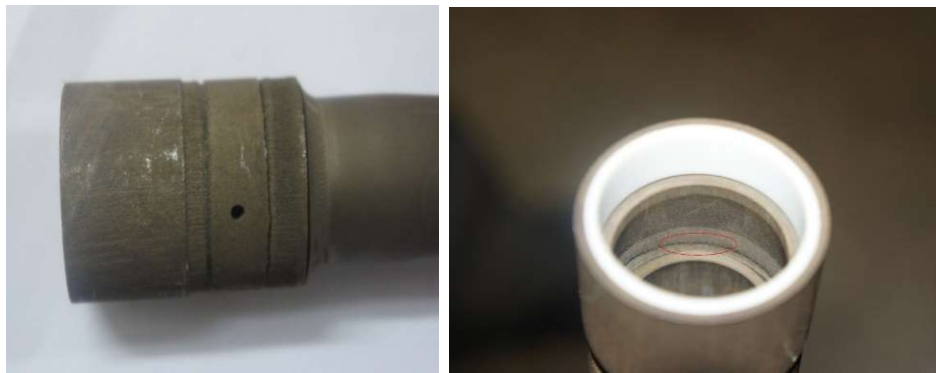
2014: Corrosion on external and internal weld seam
