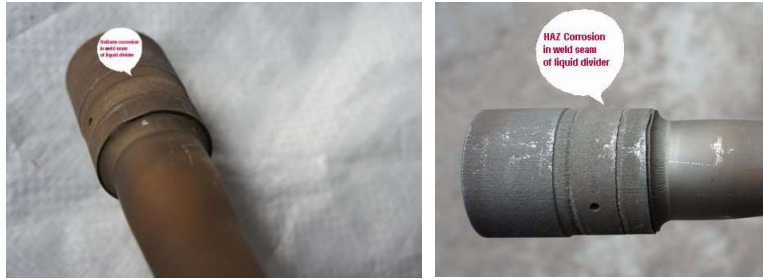
2012 : Weld seam corrosion / HAZ corrosion.
